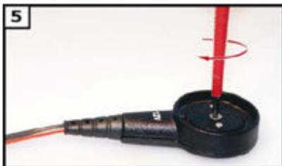
5. Close housing with screw - Ready!
